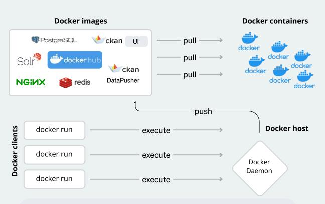
In the diagram, the Docker Host can be of any computer architecture. I personally use Mac OS for day-to-day work and Ubuntu 22.04 virtual machines for testing.
